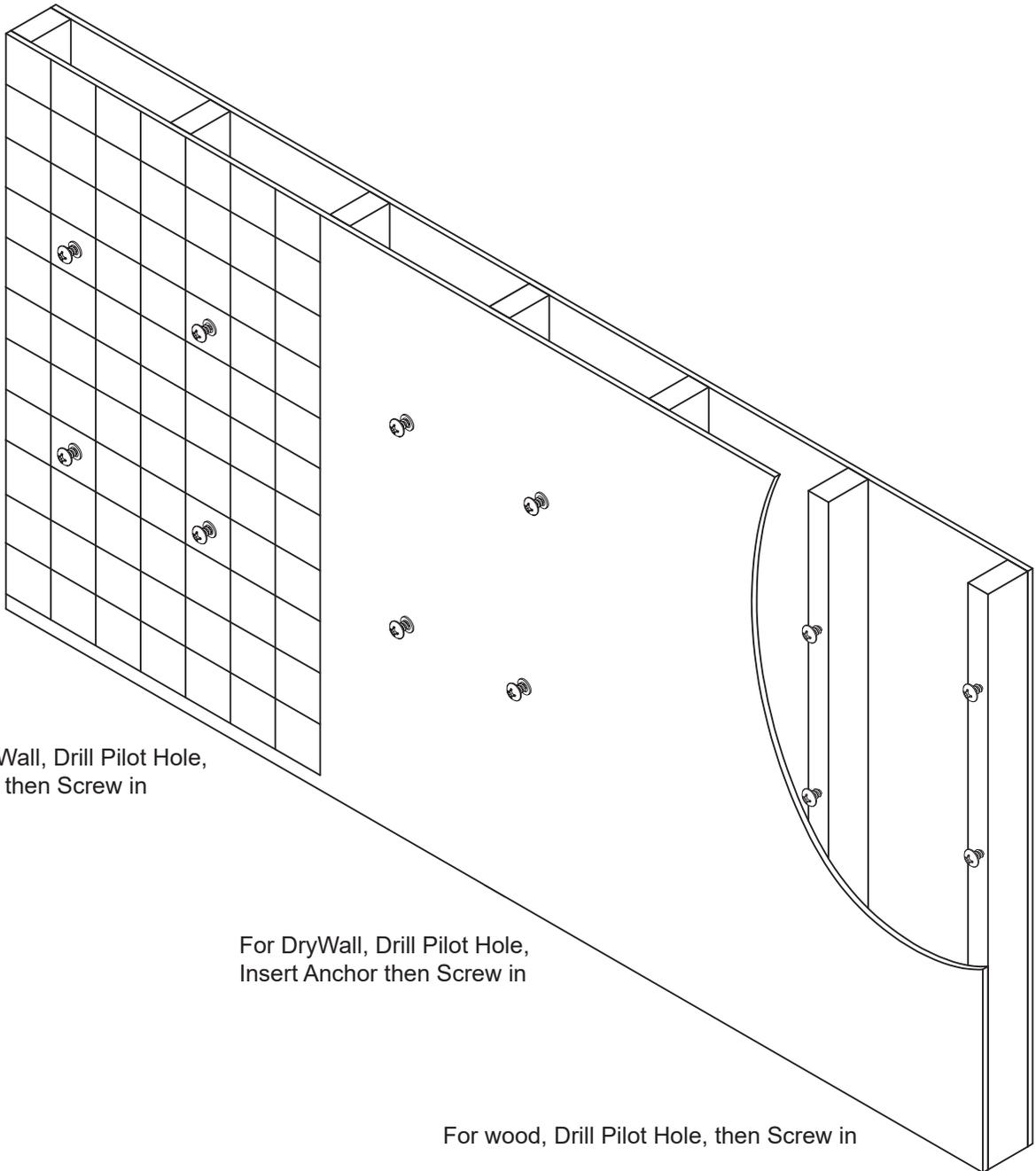
For Ceramic Wall, Drill Pilot Hole,
